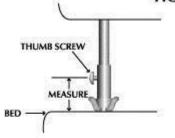
With the presser foot in the down position, measure from the BED of the machine to the center of the THUMB SCREW.
