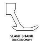
SLANT SHANK: designed ONLY for Singer slant needle machines and will NOT fit any other make of machine. Measures about 1".
